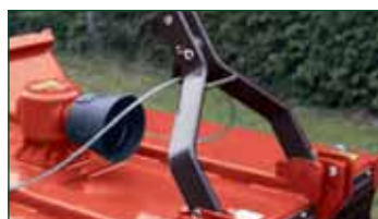
Montage attelage 3 points flottant, cat. 2
