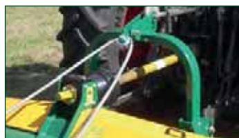
Montage attelage 3 points flottant, cat. 2
